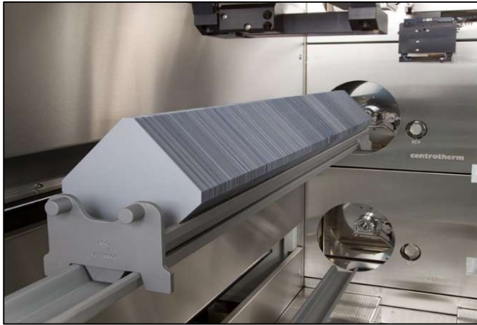
High-capacity diffusion boot with back-to-back loaded wafers
