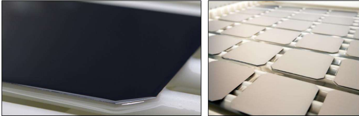
Rear Side Etching for Edge Isolation in main Etching Bath of 5-lane Industrial Inline
